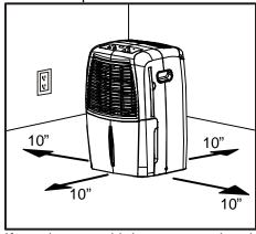
Caution: The unit is designed to be used indoors and freestanding, and not be used outdoors, or be built-in to a cabinet or used under a counter.
